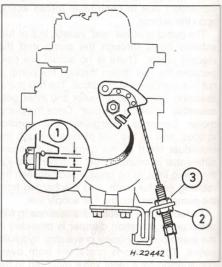
14.8 Adjust the throttle lost motion gap see text
