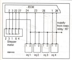
14.12 Typical local wiring diagram: injectors, stepper motor
