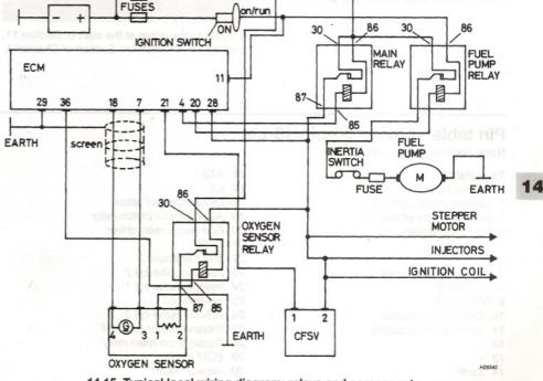
14.15 Typical local wiring diagram: relays and components
