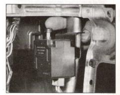
14.6 Reset inertia switch by depressing plunger
