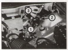
14.3 Rover 820 stepper motor 1 Stepper motor 2 Ignition coil 3 ECM
