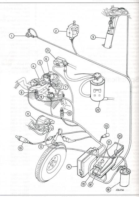
14.1 Rover MEMS (Rover 214 SPi). Multi-point systems are very similar
